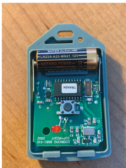
Clicker open showing battery in place. Positive is to the right.
